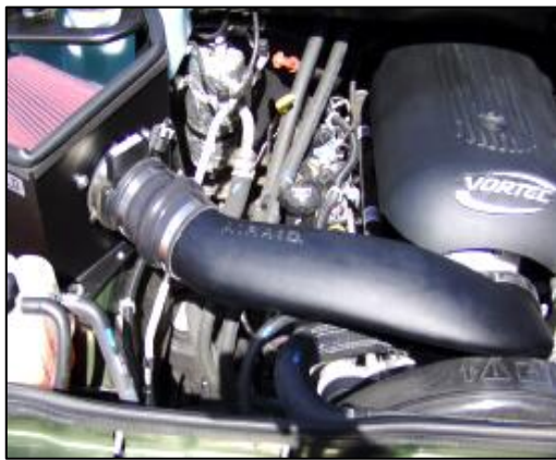
13. Connect the Airaid MIT (#5), hump hose end first, to the MAF sensor, and then connect the other end of the tube assembly to the throttle body. Check for interference and adjust the MIT accordingly, and then tighten the hose clamps.
