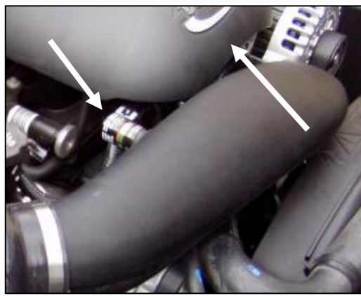
14. Re-install the factory filter minder and rubber grommet into rear of Airaid MIT. Re-install the beauty cover from step 2.
