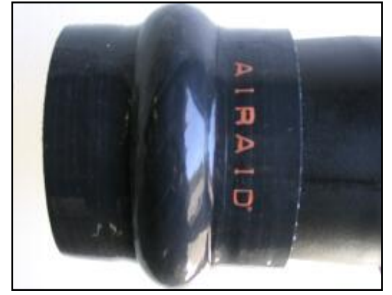
12. Install the provided urethane hump hose (#7) onto the Airaid Modular Intake Tube (MIT) (#5) with the 2 supplied #60 hose clamps (#11). Note: Leave hose clamps loose until final assembly.
