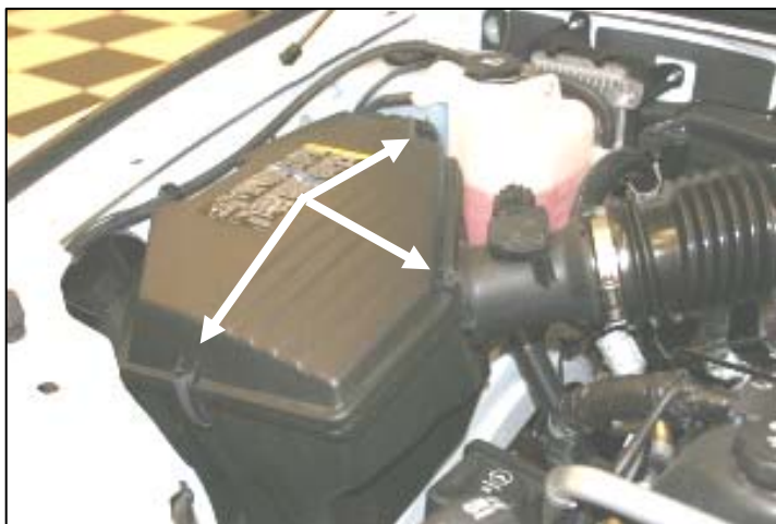
1. Disconnect the negative battery cable. Unhook the three clips that hold down the air box lid.
