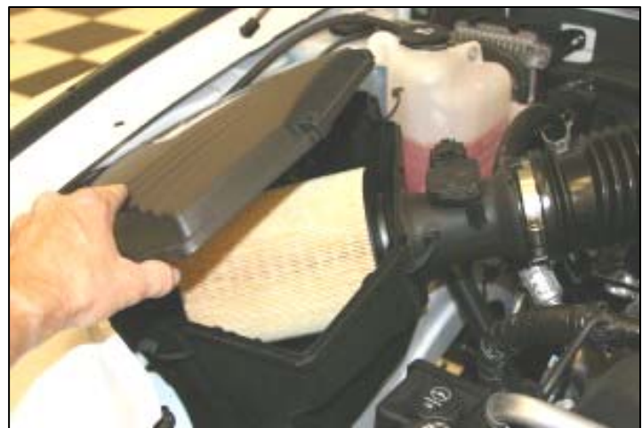
2. Remove the lid by lifting, and sliding it out of the tabs on the side of the airbox.
