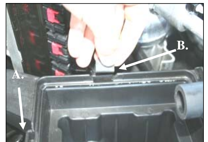
4. 2007 and newer models only: A.) Using a flat blade screwdriver, gently pry and remove one factory clip from the passenger side rear of the airbox base. (see arrow above) B.) Re-install the clip onto the rear of the factory airbox base (see arrow above).
