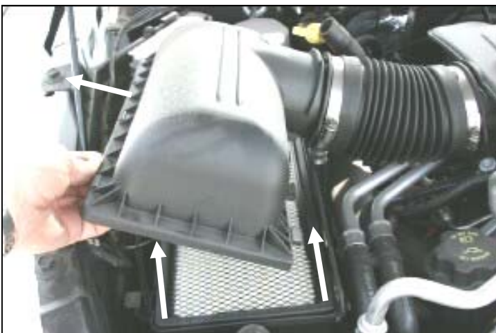
3. Remove the factory airbox lid and air filter from the airbox base.
