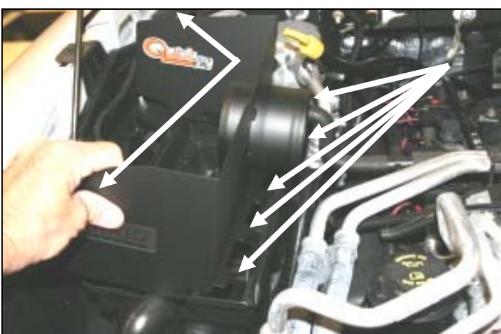
5. Slip the five tabs of the Quick fit panel (#2) through the slots on the airbox base. Adjust the panel for fit, then re-latch two of the factory clips onto the panel.
