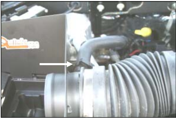
7. Re-connect the factory breather hose onto the Quick Fit Panel and secure with the #24 speed clamp (#4) as shown.
