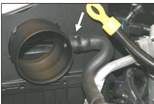
7. Re-connect the factory breather hose onto the Quick Fit Panel and secure with the #24 speed clamp (#10) as shown.
