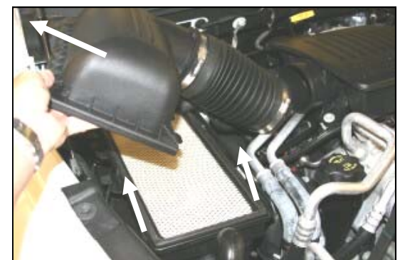
3. Remove the factory airbox lid and tube. Remove the factory air filter from the factory airbox base.
