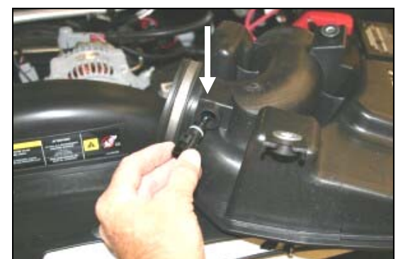
9. Carefully twist and remove the AIT sensor from the factory resonator.
