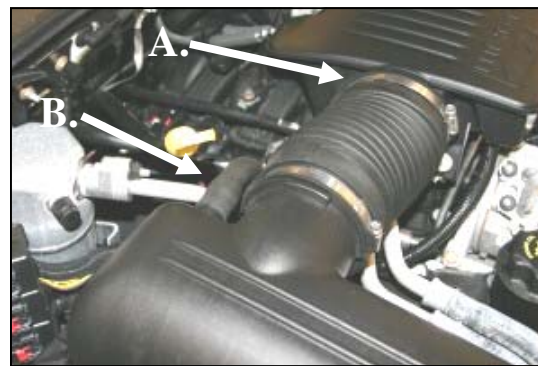
2. A.) Loosen the hose clamp on the resonator end of the intake tube. B.) Disconnect the breather hose from the factory airbox lid.
