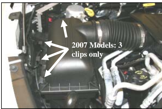
1. Disconnect the negative battery cable. Unlatch the four clips (three on 2007 models) on the factory airbox.
