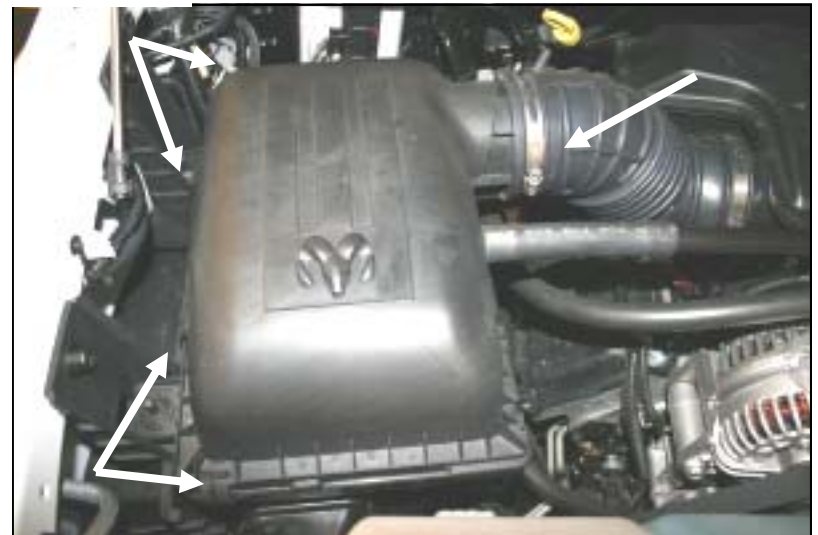
2. Unlatch 4 clips that hold down the factory airbox lid. Loosen the hose clamp on the factory intake tube where it connects to the airbox lid, then remove the lid.
