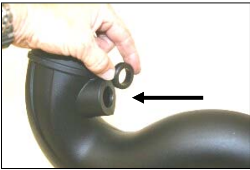
10. Install the supplied grommet (#16), into the Airaid Intake Tube (#2)
