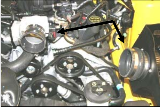
13. Install the urethane hump hose (#4) on the filter adapter (#5) with two #72 hose clamps (#13). Next install the reducing coupler (#3) small end first, onto the throttle body with one #48 hose clamp (#11), and one #52 hose clamp (#12). Leave clamps loose.
