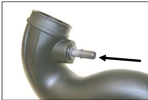
11. Install the factory fitting from step #7 into the grommet (#16) from step #10.
