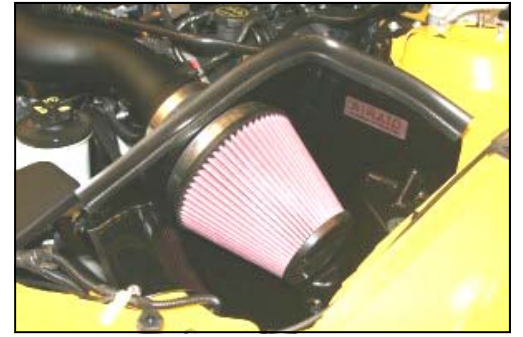
15. Install the Airaid Premium Filter (#1) onto the filter adapter (#5). Next install the weather strip (#7) on the top of the CAD as shown. Start at the front of the CAD and work towards the rear.
