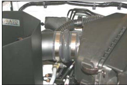
14. Center the hump hose between the tube on the factory airbox, and the tube on the CAD, adjust for fit, and tighten the hose clamps.
